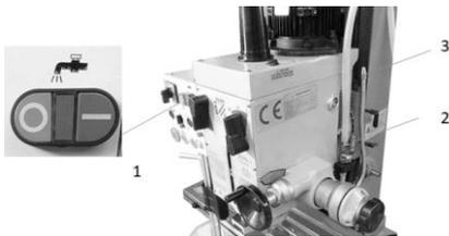
The coolant pump is switched on and off with the coolant switch (1).
