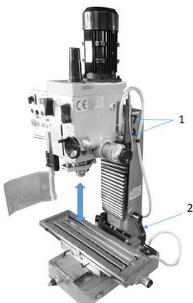
Place the provided crank handle on the shaft and secure it with the grub screw on the side.
