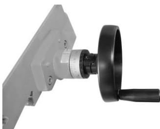
You can move the worktable in the X and Y direction to position the drill/mill in the correct position.
