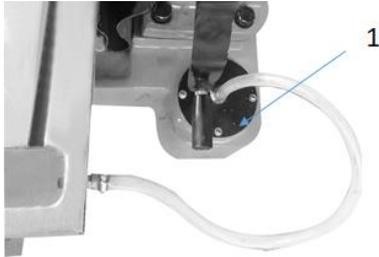
The coolant is filled into the coolant pump - see picture on the left.
