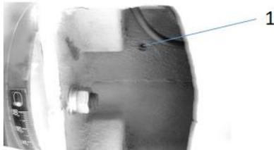
To drain the gear oil, loosen the screw (1). (Located on the underside of the gear head). Set up oil tray see note to properly catch oil. After gear oil has been completely drained. Close drain plug (1) again and fill with new gear oil.
