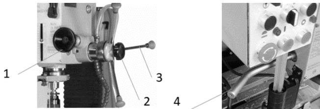
The spindle can be moved downwards/up by turning the lever (3). To do this, the fixing lever (4) must be released. The hand screw (2) is tightened for fine adjustment and the spindle lift can now be finely adjusted to the desired height using the hand wheel (1). To lock the spindle in the selected position, tighten the fixing lever (4).
