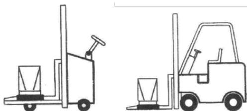
Transport the machine in its packaging to the installation site. To manoeuvre the machine in the packaging, a pallet truck or a forklift with appropriate lifting power can be used.
