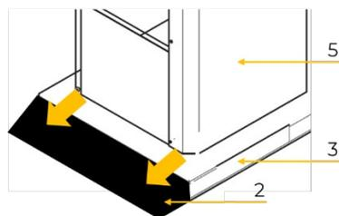
**NOTE:** Do not lift the machine at the work tables, these are not designed to withstand the tensile load of the machine weight.
