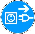
**NEVER FORGET:** Switch the machine off (38) and disconnect the machine prior to any adjustment, maintenance or check activities from the power supply. This prevents the hazard of unintended starting-up.
